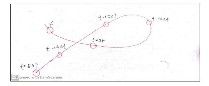
**3. Streak line:** It is an imaginary line which is passing through the points which have passed through a same point after a given time interval.
