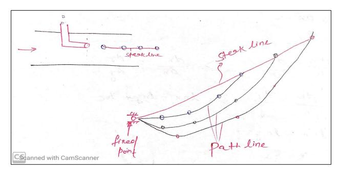
If the flow is steady, then stream line, path line and streak line will coincide.
